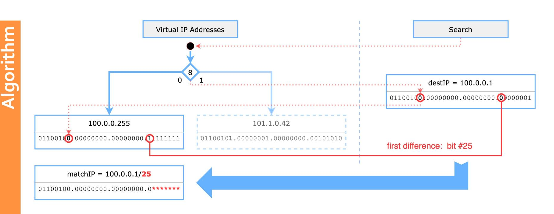
The destination IP is looked up in a Patricia Trie containing all registered virtual addresses. If the search ends up with a leaf node that does not contain the destination IP, we have a regular IP. This regular IP is then compared with the IP in the leaf node to calculate the *Unique Prefix* (shown above). By additionally using all parent prefixes to generate the IP mask, we get the Unique Mask. The generated match IP will not match any virtual address contained in the trie.
