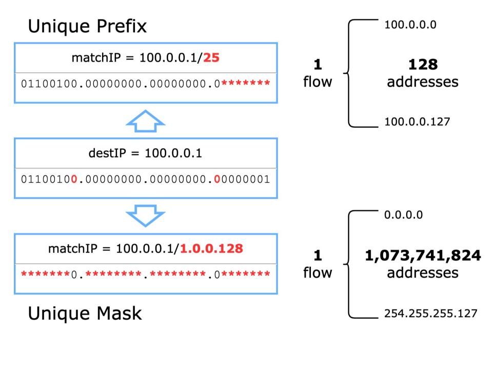
The *Unique Prefix* and the *Unique Mask* are used to generate a match IP for the switch flow. Both lead to a significant reduction in the number of flows by capturing many regular IP addresses with a single flow without also capturing a single virtual service address.
