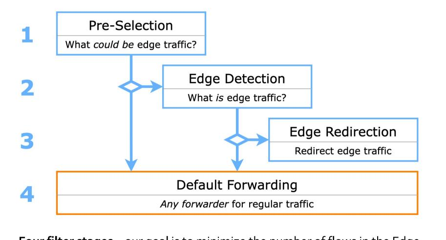
Four filter stages – our goal is to minimize the number of flows in the Edge Detection stage by matching many regular IPs with a single flow
